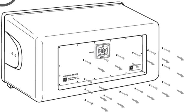
Remove screws from back plate of Control SB2210 cabinet. Keep all parts for re-assembly.
