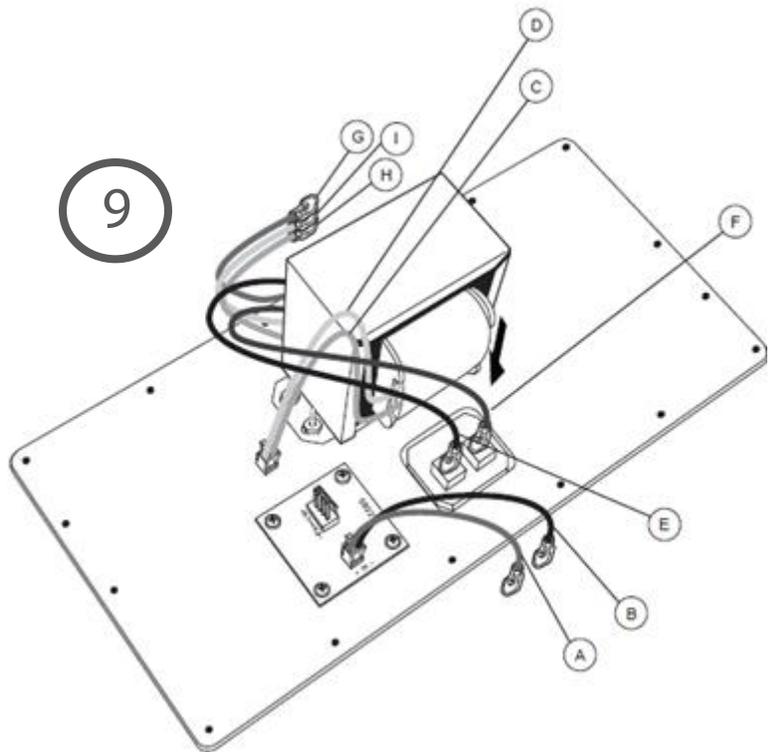
Place wire from transformer primary (F, G, H, or I) that corresponds to the desired wattage needed to tap (see chart of values on page 1) to the now open former location of the red wire (A). \*\*Please note above example shows red wire (F) connected to input PC board which is the 300W tap for 70V use.
