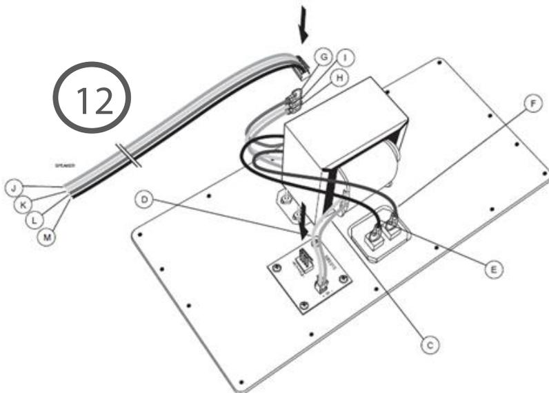
Reattach large multi-pin connector from the (2) woofers to the PC board as shown in above drawing.
