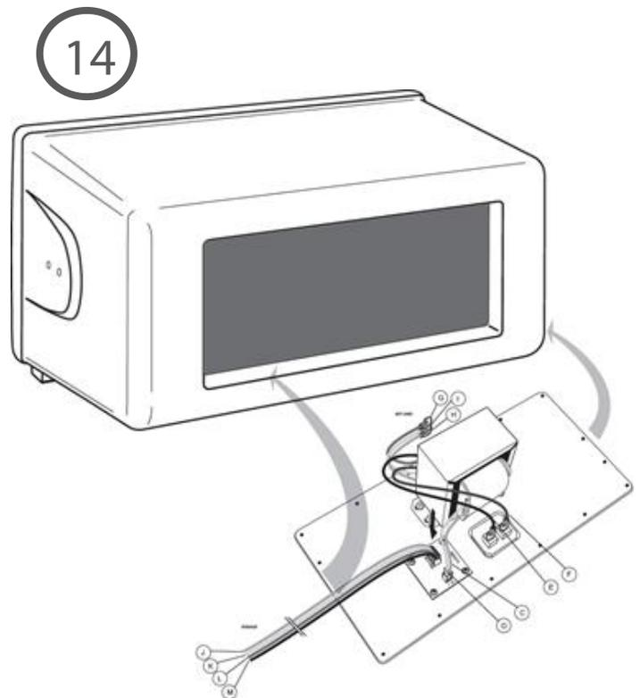
Replace back panel onto back of enclosure and tighten down plate firmly with original screws.
