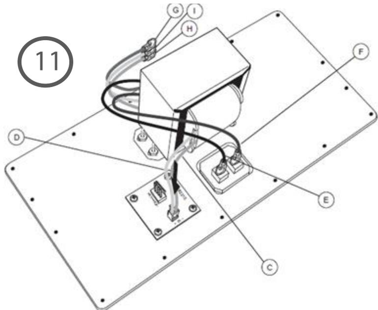
Attach yellow wire (D) and green wire (C) to the now open former location of the connector from the red wire (A) and black wire (B). This is the location for the positive "+" and negative "-" wires from the transformer secondary.
