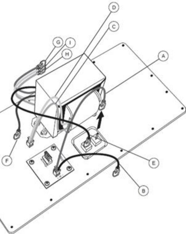
Remove red wire (A) from input PC board as shown in above drawing.
