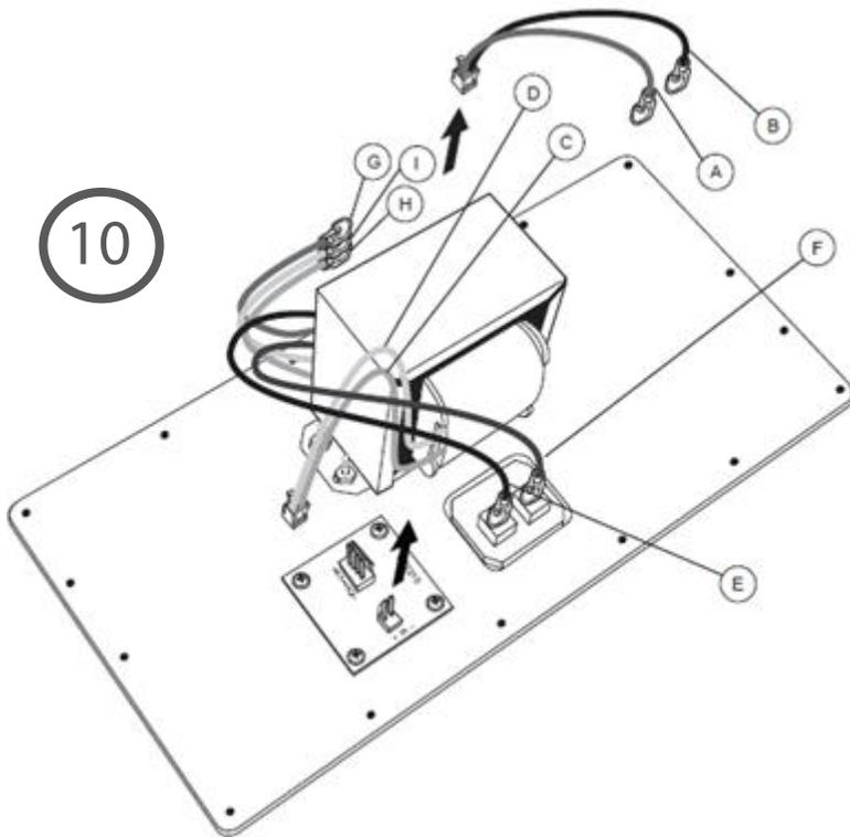
Unplug connector attached to the end of the red wire (A) and black wire (B) from the PC board and set aside. This cable connection is no longer needed for use with the transformer.
