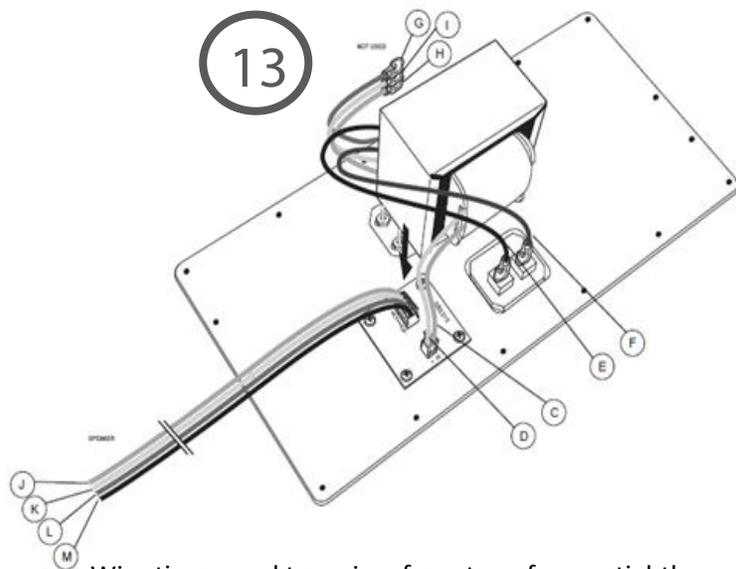
Wire tie unused tap wires from transformer tightly so Conductive parts cannot contact each other or other parts and so that they can't rattle with vibration.
